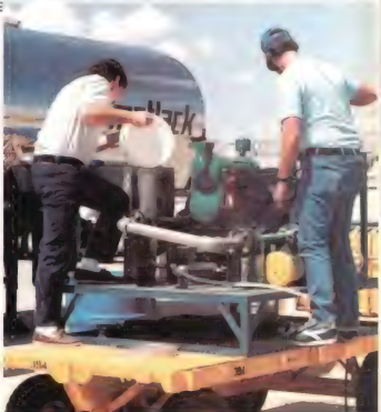
Fire retardant: an experimental additive is mixed with regular jet fuel
